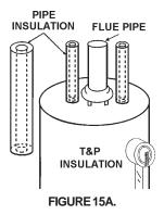
Fit pipe insulation over the incoming cold water line and the hot water line. Make sure that the insulation is against the top cover of the heater.
